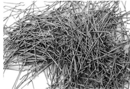
Fig. 1. Steel fiber (SF) used in this study
