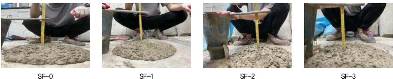
Fig. 4. Slump test for fresh RWM
