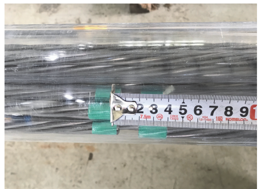
Fig. 5 2 cm of 2 strands damage case
