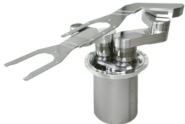
[Fig. 1] A wafer transfer robot that residual vibrations should be suppressed as quickly as possible in point-to-point motions. (Courtesy of Hirata Corporation)
