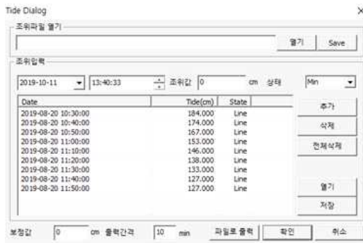
FIGURE 15. Loading tide level data in 10minute increments (See FIGURE 6)
