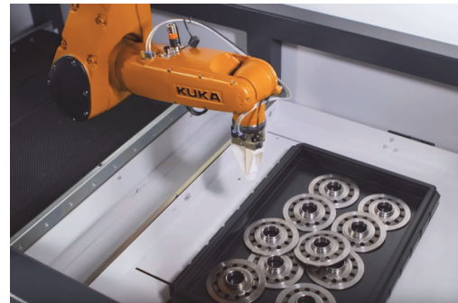
(a) Experimental setup for bin-picking
