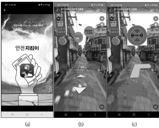
Fig. 11. AR based smartphone application for evacuating the infected area (a) Homepage screen shot of the proposed application, (b) A screen that informs the risk of infection when the elderly are in an alerting area, (c) A screen that informs the evacuation route when the elderly are in a warning area
