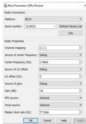
Figure 7: Programming USRP via Simulink
