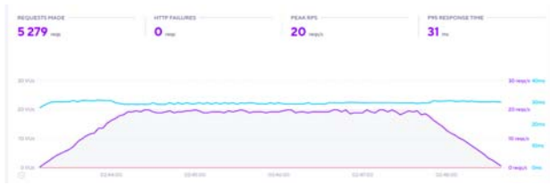
Fig. 9 Scenario 1 Normal Traffic Without Firewall.
