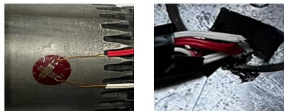
(b) Strain gauge wiring picture
