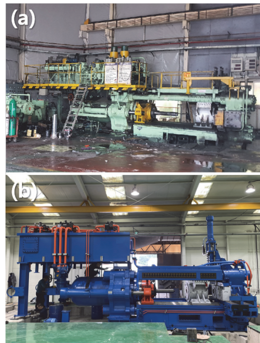
Fig. 2 Before(a) and after(b) extruder remanufacturing
