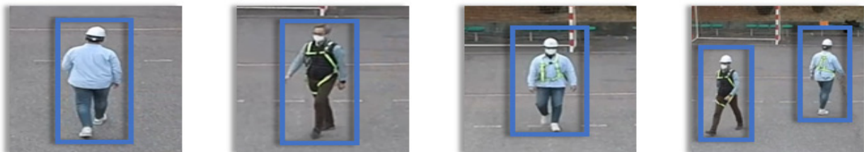
Figure 4. Worker detection through YOLO-v3
