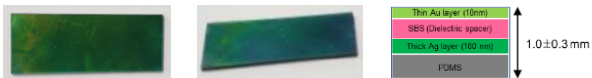
Figure 1. Shape and structure of mechanochromic sensor
