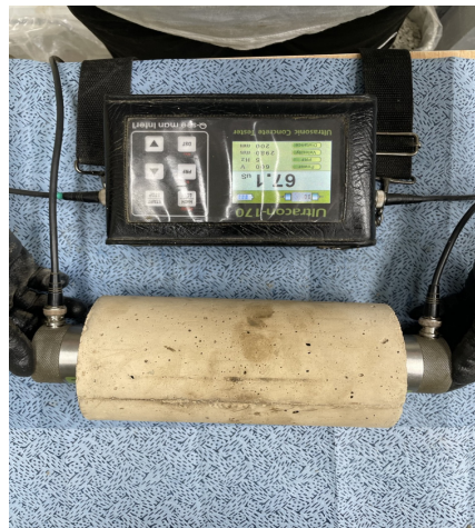
Figure 3. Ultrasonic pulse velocity test
