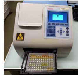
Fig. 1-3. Measure the absorbance of water and 50% ethanol extracts for each sample with a microplate reader at wavelengths for each color band
