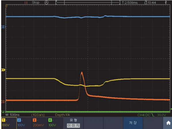
Fig. 5. The measurement of the light waveform of the write discharge during the write period in the modified single sustain driving method.
