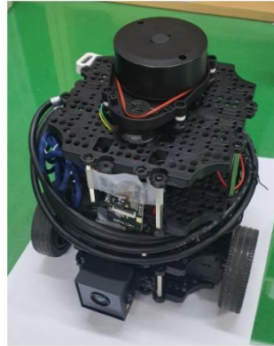
Figure 2. Turtlebot 3 burger used to collect data for REM construction
