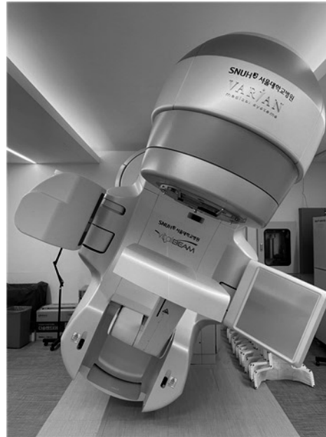
Fig. 1. Linear accelerator and electronic portal imaging device for portal dosimetry. Source to imager distance = 100 cm.
