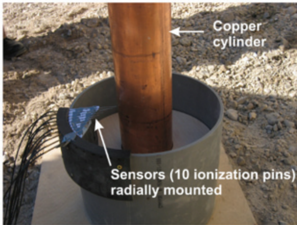
Fig. 5. Cylinder test arrangement (Esen et al., 2005 and Sanchidrian et al., 2015).
