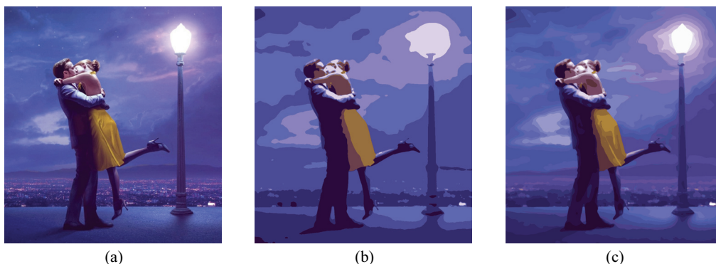
Fig. 3. Example of color clustering: (a) source image, (b) image clustered in eight colors, and (c) image clustered in 32 colors.
