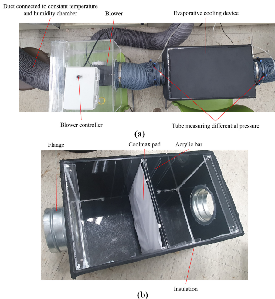
Figure 2. Experimental setup: (a) Experimental device, (b) Evaporative cooling device and cooling pad.
