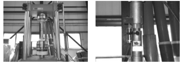
(a) Cyclic loading test setup
