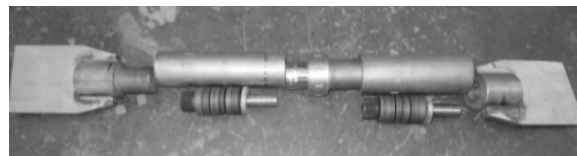
(b) Specimen (Spring stack)
