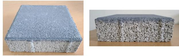
Fig. 1. The specimens of concrete sidewalk blocks
