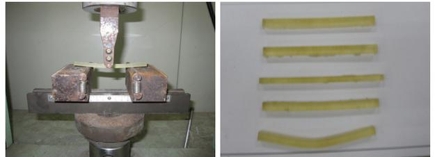
Fig. 5. Flexural strength test and specimen shape
