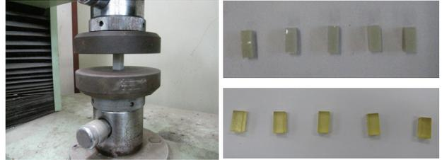
Fig. 4. Compressive strength test and specimen shape
