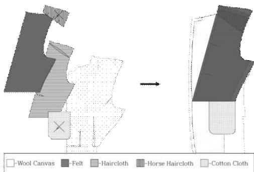
<Fig. 18> Non-adhesive fabrication method chest canvas
