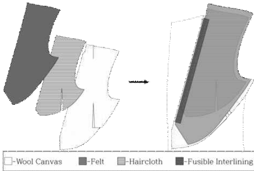
<Fig. 10> Adhesive fabrication method chest canvas
