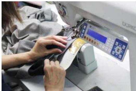
<Fig. 12> Adhesive fabrication method sleeve attachment
