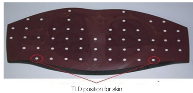
Fig. 2. A layer of the torso part of the Alderson-Rando phantom and the location of the thermoluminescent dosimeters (TLDs).
