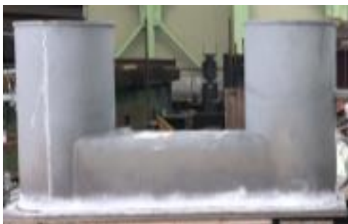
(b) typical bollard with two columns
