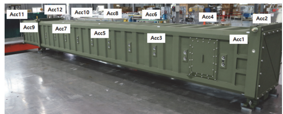
Fig. 5. Sensor mount positions for modal analysis of similar vertical launch vehicle
