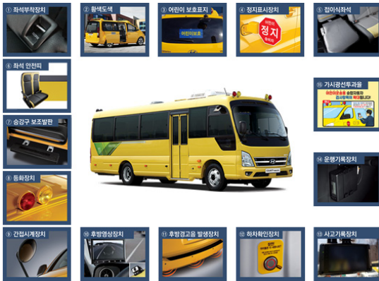
Fig. 1 School bus mandatory installation device
