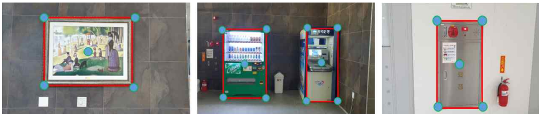
FIGURE 11. Characteristic landmark location information of corners and center points for image localization
