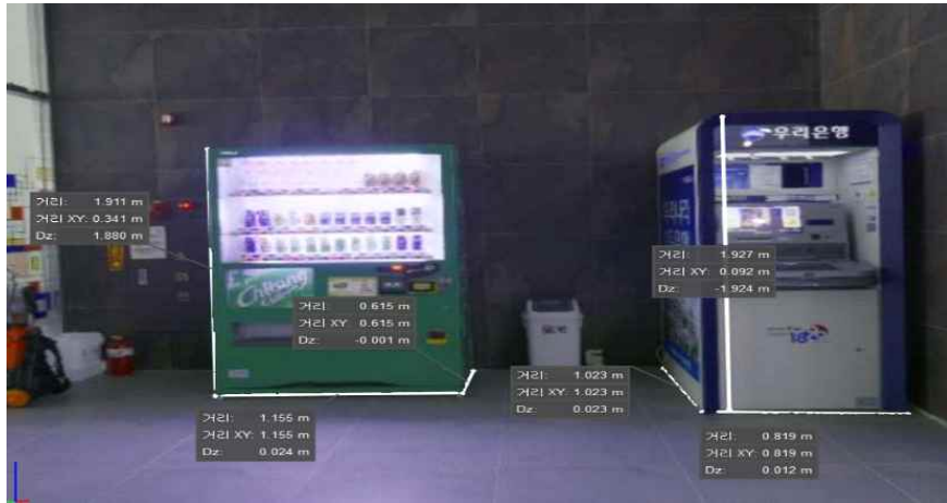
FIGURE 10. Precise 3D length and coordinates measuring between terrestrial LiDAR point cloud
