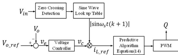
Fig. 5. Block diagram of predictive current mode control.
