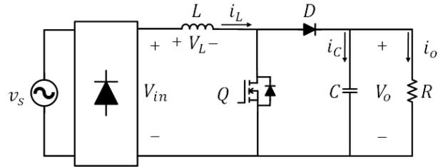
Fig. 1. Circuit diagram of single-phase Boost PFC converter.
