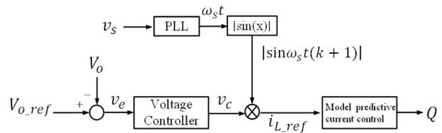
Fig. 6. Block diagram of model predictive current control.
