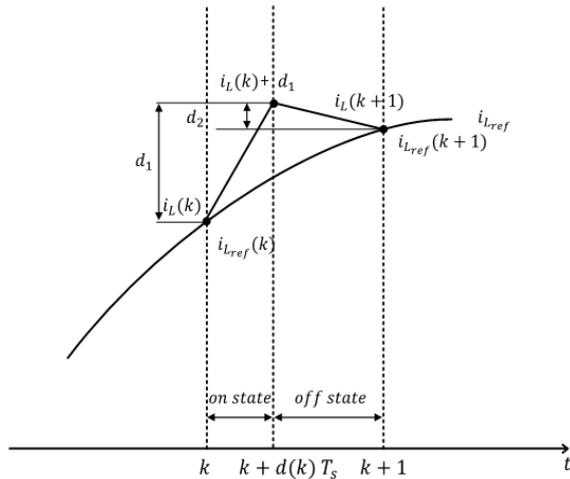
Fig. 4. Operation principle of predictive current mode control.
