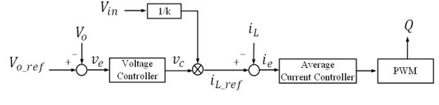
Fig. 3. Block diagram of average current mode control.
