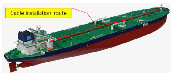
Fig. 6 An example of the deck section where cables are installed in a straight line on the ship
