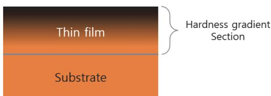
**Fig. 4.** Functional Graded Material structure by IPL.
