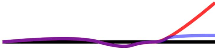
Fig. 1. Over-estimation and under-estimation problem of pixel-based performance evaluation (Black line depicts ground truth. Blue line and red line depicts the model A and the model B. In this case, the evaluation metric will be almost identical, so the performance of the model A is over-estimated, and vice versa.)
