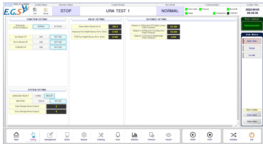
Fig. 9. Set the motor speed of clean roll
