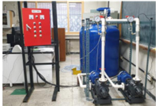
Fig. 2. Experiment setups of fire pumps.
