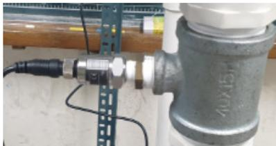
Fig. 5. Pressure sensor of PT-506.
