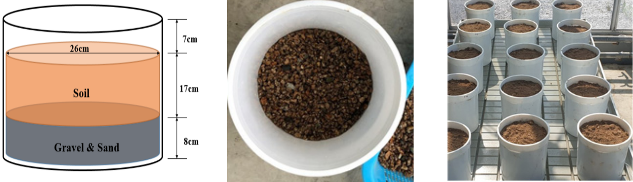
Fig. 1. Diagram for the soil layers in the wagner pot.
