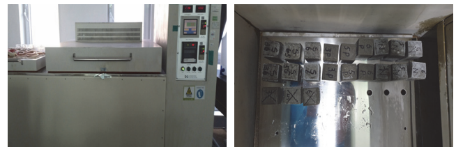
Fig. 5 View of freezing and thawing resistance test
