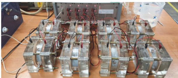
Fig. 6 View of chloride penetration resistance test
