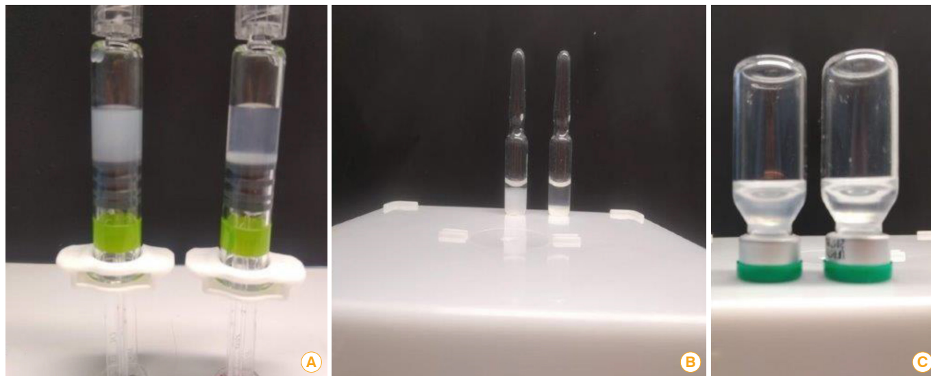
Fig. 4. Example of non-frozen (left side) and frozen (right side) vaccines packed in the different types of containers after 10 minutes from shaking for 10 seconds. (A) The pre-filled syringe. (B) The ampoule. (C) The vial.
