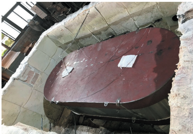
Fig. 4. Photograph of the test model installed in the furnace.
