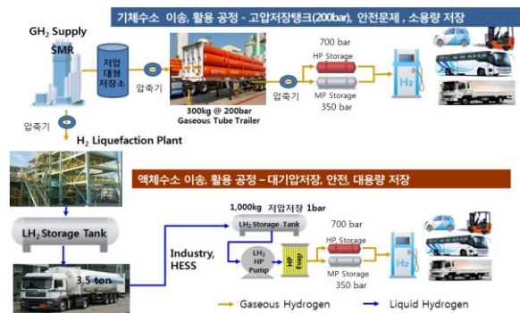
Fig. 1. Hydrogen station supply system schematic diagram [6].
