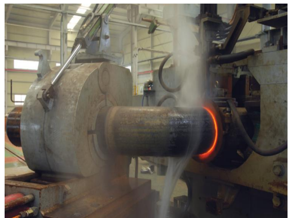
Fig. 2 Equipment of induction bending
