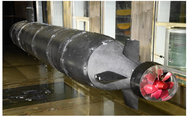
Fig. 9 Installation for the self-propulsion test
