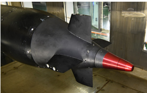
Fig. 5 Setup for bare hull resistance test
