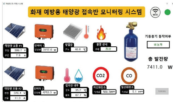
Fig. 6. Python monitoring system of photovoltaic connection module.
