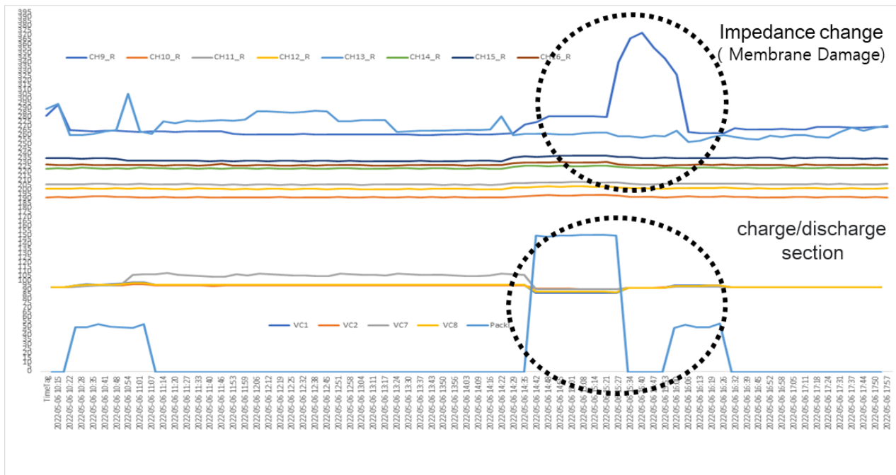
Figure 5. Change of impedance value measured for each cell using battery diagnostic module device
