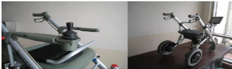
Figure 9. The final concept product of the proposed 3-stage folding electric kickboard
