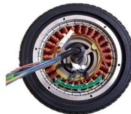
Figure 3. Adopted In Wheel Outer Rotor method
