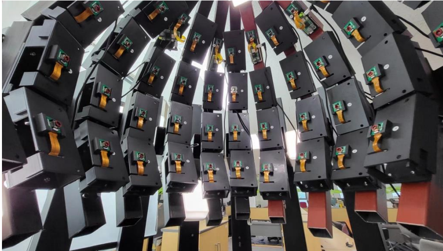
Figure 6. Second self-made camera array
