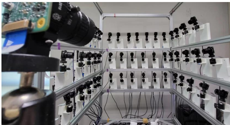
Figure 3. First self-made camera array layout
