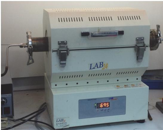
Fig. 2 Tube furnace reactor
