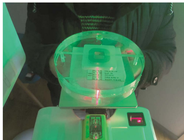
Fig. 2. A dental volume tomography phantom is positioned using a fabricated mounting table with a flat top. The center of the phantom is positioned at the center of the field of view of the cone-beam computed tomography device.
