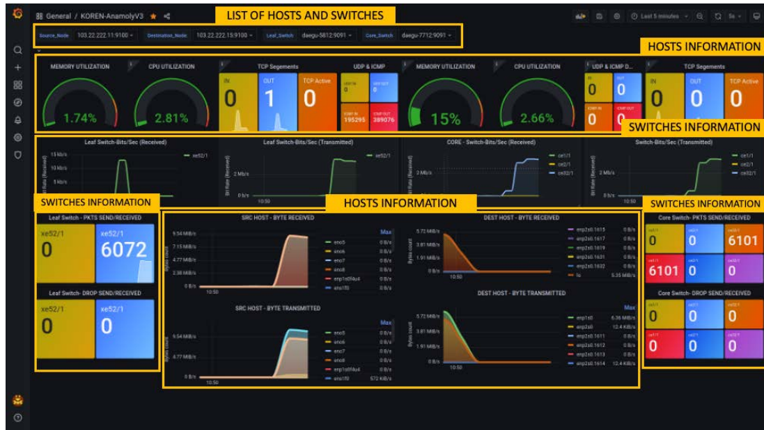
Fig. 4. Grafana Dashboard: with dropdown list of host and switch, the host resource utilization information such as memory and CPU, and switches traffic information such bytes and packets count.
