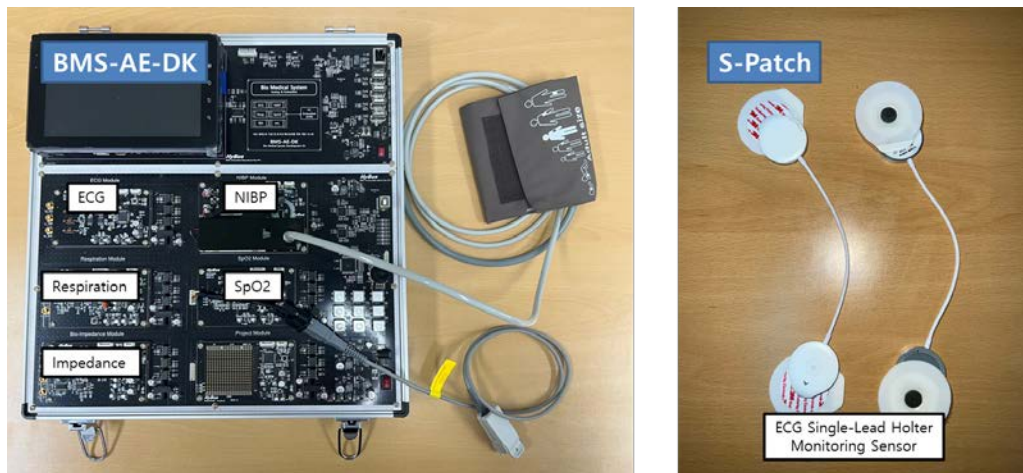
Fig. 6. BMS-AE-DK biometric sensor and S-Patch ECG sensors in smart space device part
